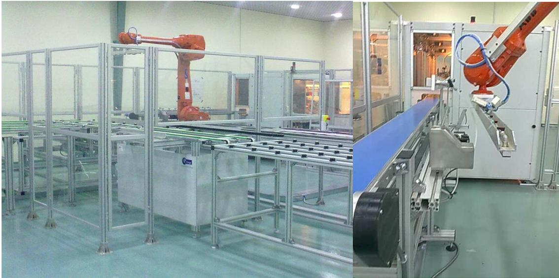
The automatic layup station **P.ENERGY LO072AR** is a robotic system that takes the strings of cells from the Tabber&Stringer machines and places them correctly aligned onto the glass.
